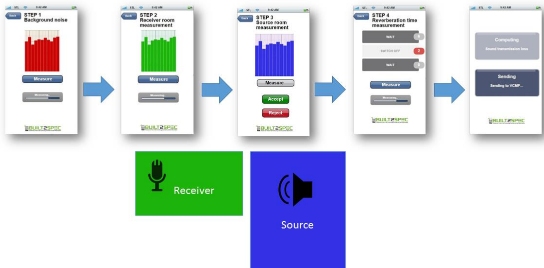
Figure: Workflow acoustic tool
