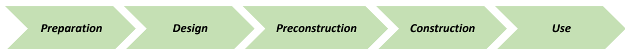
Fig. 4 Typical example of main stages of a European construction process with tender (e.g. RIBA work stages)
