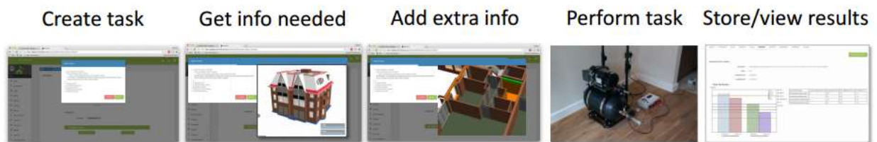
Figure 4.1 : The generic use-case in Built2Spec (using an example of the air tightness test)
