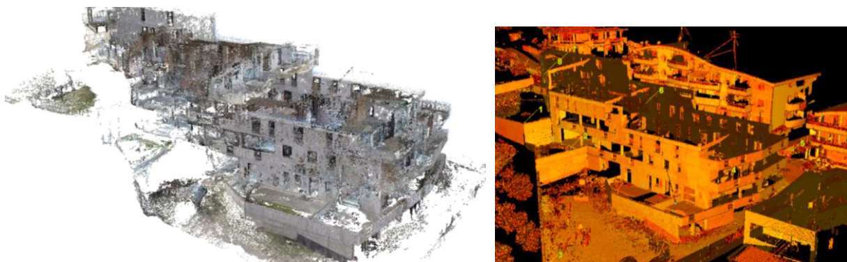
Figure 4-6 3D Reconstruction from GoPro images using COLMAP (left) and Leica Scanner (right).
