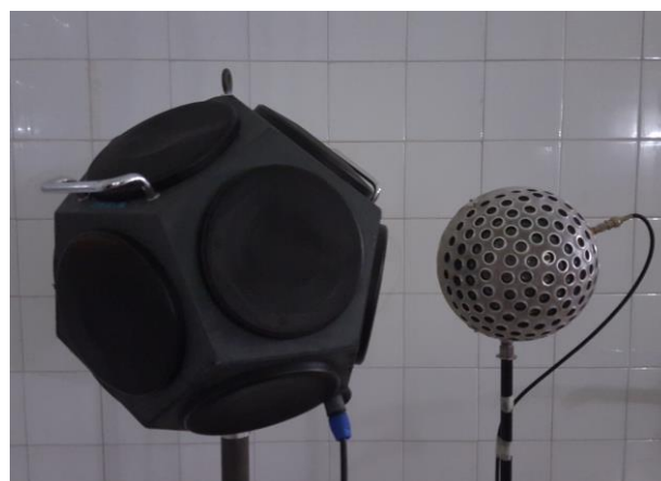
Figure 2.1. (Right) Standard omnidirectional sound source and (left) proposed omnidirectional parametric loudspeaker (OPL).
