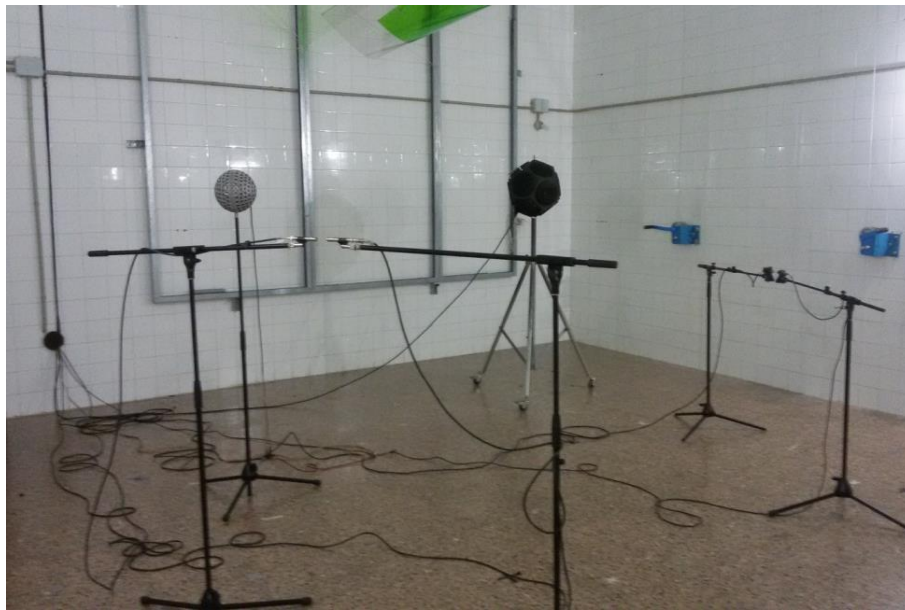
Figure 4.4. Experimental setup within the reverberant chamber. Two pairs of microphones and sound sources (OPL#1 and CESVA) distributed randomly in the chamber.
