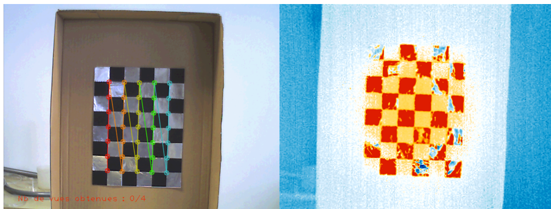
Figure 43: Left: OpenCV checkerboard detection using a custom checkerboard made out of reflective tape. Right: Detection failure using the thermal image.
