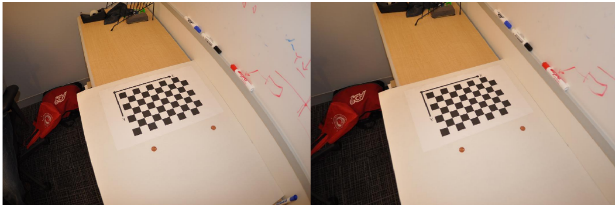
Figure 39: Distortion removal from an image. (Left) Original image captured with a camera. (Right) Undistorted image. Note the bottom of the whiteboard that is curved in the left (original) image and straight in the right (rectified) image. Source MathWorks 9
