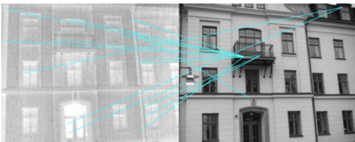
Figure 45: Corresponding SIFT features from two images of the same building. Left: Thermal image. Right: RGB image. The blue lines represent the computed correspondences between keypoints extracted from the thermal and the RGB images. One can observe that many of these correspondences are false (a keypoint in the thermal image does not correspond to the same point in the RGB image). Source (Liu et Seipel 2015).
