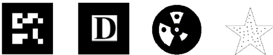
Figure 37: Examples of fiducial markers used in Augmented Reality. From left to right: ARTag (Fiala 2005) marker, ARToolKit (Kato et Billingham 1999) marker, Circular Marker (Naimark et Foxlin 2002) and Random Dot Marker (Uchiyama et Saito 2011).
