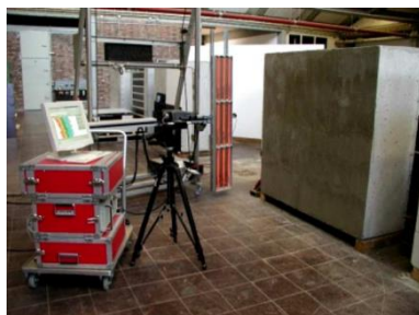
Fig.26 (Left) Experimental set-up; (Right) Concrete test specimen with voids (units are in cm)
