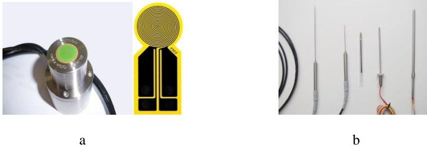
Fig 8 Heating sources a. disc; b. needle probe
