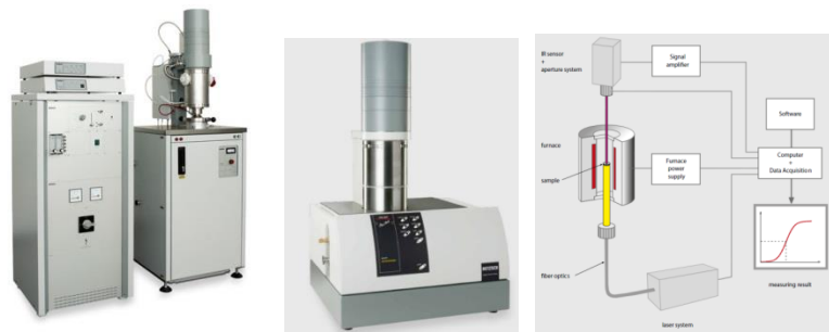
Fig.11 Instrument of NETZSCH and its principle based on Flash method
